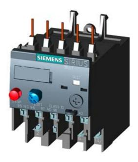
OVERLOAD RELAY 4.5...6.3 A FOR MOTOR PROTECTION SZ S00, CLASS 10, F. MOUNTING ONTO CONTACTOR MAIN CIRCUIT: RING CABLE LUG AUX. CIRCUIT: RING CABLE LUG MANUAL-AUTOMATIC-RESET
