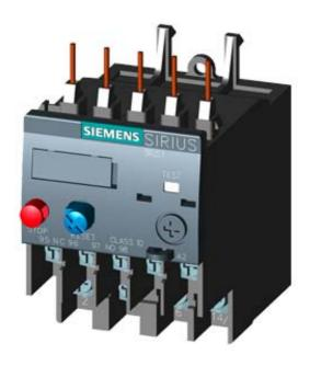
OVERLOAD RELAY 2.8...4.0 A FOR MOTOR PROTECTION SZ S00, CLASS 10, F. MOUNTING ONTO CONTACTOR MAIN CIRCUIT: RING CABLE LUG AUX. CIRCUIT: RING CABLE LUG MANUAL-AUTOMATIC-RESET
