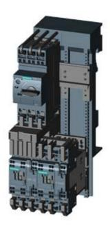
LOAD FEEDER FUSELESS REVERSING DUTY, AC 400V, SZ S0, 14. . .20A, AC 230V SPRING-LOADED TERMINAL FOR BUSBAR SYSTEMS 60MM TYPE OF COORDINATION 1, IQ = 150KA 1NO+1NC (CONTACTOR)
