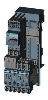
LOAD FEEDER FUSELESS REVERSING DUTY, AC 400V, SZ S0, 11...16A, AC 230V SPRING-LOADED CONNECTION FOR BUSBAR SYSTEMS 60MM TYPE OF COORDINATION 2, IQ = 150KA (ALSO FULFILLS TYPE OF COORDINATION 1) 1NO+1NC (CONTACTOR)
