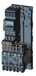
LOAD FEEDER FUSELESS REVERSING DUTY, AC 400V, SZ S0, 11...16A, AC 230V SPRING-LOADED CONNECTION FOR RAIL-MOUNTING, W. DIN RAIL ADAPTER TYPE OF COORDINATION 2, IQ = 150KA (ALSO FULFILLS TYPE OF COORDINATION 1)
