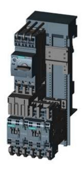
LOAD FEEDER FUSELESS REVERSING DUTY, AC 400V, SZ S0, 27...32A, DC 24V SPRING-LOADED CONNECTION FOR BUSBAR SYSTEMS 60MM TYPE OF COORDINATION 2, IQ = 150KA (ALSO FULFILLS TYPE OF COORDINATION 1) 1NO+1NC (CONTACTOR)
