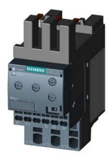
MONITORING RELAY ATTACHABLE TO CONTACTOR 3RT2. SIZE S0 BASIC, ANALOG ADJUSTABLE APPARENT CURRENT MONITORING 4 - 40A, 50-60 HZ, 2-PHASE SUPPLY 24-240 V AC/DC 1 CO CONTACT MONITORING FOR CURRENT OVERSHOOT/UNDERSHOOT PHASE FAILURE, WIRE BREAK WITH OR W/O ERROR LOG ON-DELAY 0-60 S SPURIOUS PEAK SUPPR.0-30 S SWITCHING HYSTERESIS 6% SPRING-LOADED CONNECTION
