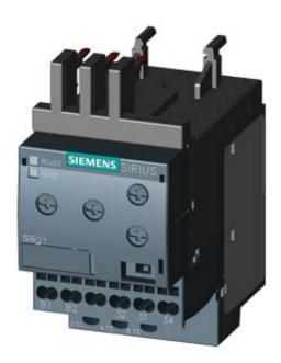
MONITORING RELAY ATTACHABLE TO CONTACTOR 3RT2. SIZE S00 BASIC, ANALOG ADJUSTABLE APPARENT CURRENT MONITORING 1.6 - 16A, 50-60 HZ, 2-PHASE SUPPLY 24 V AC/DC 1 CO CONTACT MONITORING FOR CURRENT OVERSHOOT/UNDERSHOOT PHASE FAILURE, WIRE BREAK WITH OR W/O ERROR LOG ON-DELAY 0-60 S SPURIOUS PEAK SUPPR.0-30 S SWITCHING HYSTERESIS 6% SPRING-LOADED CONNECTION
