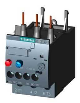
OVERLOAD RELAY 5.5...8.0 A FOR MOTOR PROTECTION SZ S0, CLASS 10, F. MOUNTING ONTO CONTACTOR MAIN CIRCUIT: SCREW TERMINAL AUX. CIRCUIT: SCREW TERMINAL
