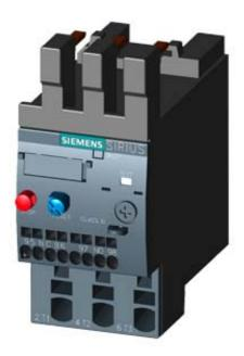
OVERLOAD RELAY 9.0...12.5 A FOR MOTOR PROTECTION BGR S0, CLASS 10 FOR MOUNTING ONTO CONTACTORS MAIN CIRCUIT: SPRING-LOADED TERMINAL AUXILARY CIRCUIT:SPRING-LOADED TERMINAL MANUAL-AUTOMATIC-RESET
