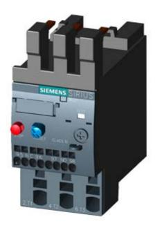
OVERLOAD RELAY 4.5...6.3 A FOR MOTOR PROTECTION SZ S0, CLASS 10, F. MOUNTING ONTO CONTACTOR MAIN CIRCUIT: SPRING TERMINAL AUX. CIRCUIT: SPRING TERMINAL
