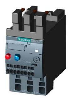
OVERLOAD RELAY 2.8...4.0 A FOR MOTOR PROTECTION SZ S0, CLASS 10, F. MOUNTING ONTO CONTACTOR MAIN CIRCUIT: SPRING TERMINAL AUX. CIRCUIT: SPRING TERMINAL MANUAL-AUTOMATIC-RESET
