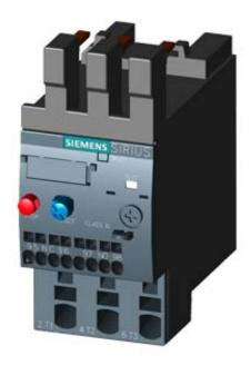
OVERLOAD RELAY 2.2...3.2 A FOR MOTOR PROTECTION SZ S0, CLASS 10, F. MOUNTING ONTO CONTACTOR MAIN CIRCUIT: SPRING TERMINAL AUX. CIRCUIT: SPRING TERMINAL MANUAL-AUTOMATIC-RESET
