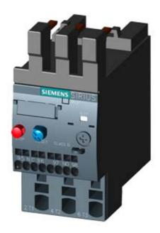
OVERLOAD RELAY 1.8...2.5 A FOR MOTOR PROTECTION SZ S0, CLASS 10, F. MOUNTING ONTO CONTACTOR MAIN CIRCUIT: SPRING TERMINAL AUX. CIRCUIT: SPRING TERMINAL
