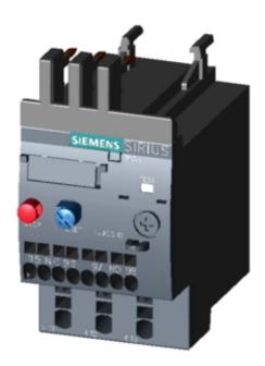
OVERLOAD RELAY 7.0...10 A FOR MOTOR PROTECTION SZ S00,
