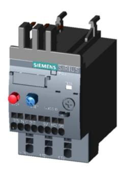
OVERLOAD RELAY 3.5...5.0 A FOR MOTOR PROTECTION SZ S00, CLASS 10, F. MOUNTING ONTO CONTACTOR MAIN CIRCUIT: SPRING TERMINAL AUX. CIRCUIT: SPRING TERMINAL
