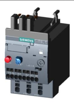
OVERLOAD RELAY 2.8...4.0 A FOR MOTOR PROTECTION SZ S00, CLASS 10, F. MOUNTING ONTO CONTACTOR MAIN CIRCUIT: SPRING TERMINAL AUX. CIRCUIT: SPRING TERMINAL
