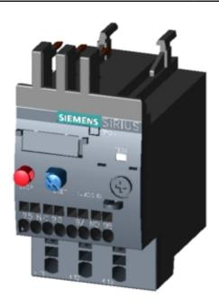
OVERLOAD RELAY 1.8...2.5 A FOR MOTOR PROTECTION SZ S00, CLASS 10, F. MOUNTING ONTO CONTACTOR MAIN CIRCUIT: SPRING TERMINAL AUX. CIRCUIT: SPRING TERMINAL
