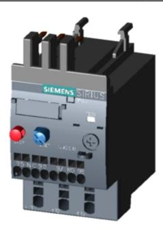
OVERLOAD RELAY 1.4...2.0 A FOR MOTOR PROTECTION SZ S00, CLASS 10, F. MOUNTING ONTO CONTACTOR MAIN CIRCUIT: SPRING TERMINAL AUX. CIRCUIT: SPRING TERMINAL MANUAL-AUTOMATIC-RESET
