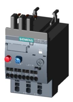
OVERLOAD RELAY 0.45...0.63 A FOR MOTOR PROTECTION SZ S00, CLASS 10, F. MOUNTING ONTO CONTACTOR MAIN CIRCUIT: SPRING TERMINAL AUX. CIRCUIT: SPRING TERMINAL
