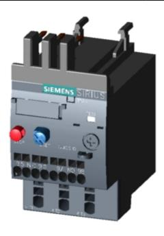
OVERLOAD RELAY 0.35...0.50 A FOR MOTOR PROTECTION SZ S00, CLASS 10, F. MOUNTING ONTO CONTACTOR MAIN CIRCUIT: SPRING TERMINAL AUX. CIRCUIT: SPRING TERMINAL MANUAL-AUTOMATIC-RESET
