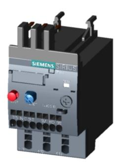
OVERLOAD RELAY 0.28...0.40 A FOR MOTOR PROTECTION SZ S00, CLASS 10, F. MOUNTING ONTO CONTACTOR MAIN CIRCUIT.
