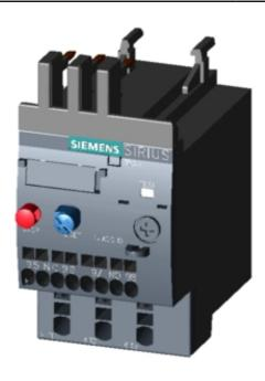
OVERLOAD RELAY 0.18...0.25 A FOR MOTOR PROTECTION SZ S00, CLASS 10, F. MOUNTING ONTO CONTACTOR MAIN CIRCUIT: SPRING TERMINAL AUX. CIRCUIT: SPRING TERMINAL MANUAL-AUTOMATIC-RESET
