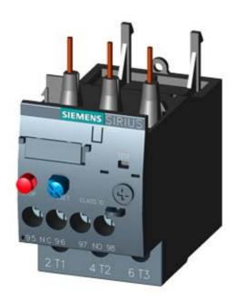
OVERLOAD RELAY 9.0...12.5 A FOR MOTOR PROTECTION BGR S00, CLASS 10 FOR MOUNTING ONTO CONTACTORS MAIN CIRCUIT:SCREW TERMINAL AUXILARY CIRCUIT:SCREW TERMINAL MANUAL-AUTOMATIC-RESET
