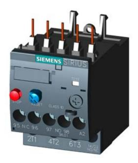
OVERLOAD RELAY 1.1...1.6 A FOR MOTOR PROTECTION SZ S00, CLASS 10, F. MOUNTING ONTO CONTACTOR MAIN CIRCUIT: SCREW TERMINAL AUX. CIRCUIT: SCREW TERMINAL MANUAL-AUTOMATIC-RESET
