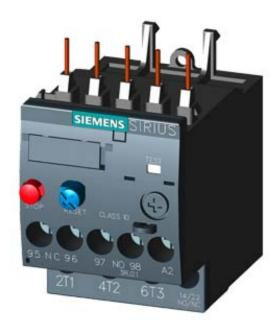
OVERLOAD RELAY 0.45...0.63 A FOR MOTOR PROTECTION SZ S00, CLASS 10, F. MOUNTING ONTO CONTACTOR MAIN CIRCUIT: SCREW TERMINAL AUX. CIRCUIT: SCREW TERMINAL MANUAL-AUTOMATIC-RESET
