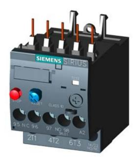
OVERLOAD RELAY 0.18...0.25 A FOR MOTOR PROTECTION SZ S00, CLASS 10, F. MOUNTING ONTO CONTACTOR MAIN CIRCUIT: SCREW TERMINAL AUX. CIRCUIT: SCREW TERMINAL MANUAL-AUTOMATIC-RESET
