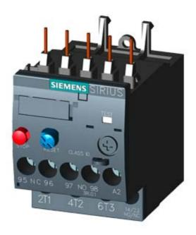
OVERLOAD RELAY 0.14...0.20 A FOR MOTOR PROTECTION SZ S00, CLASS 10, F. MOUNTING ONTO CONTACTOR MAIN CIRCUIT:
