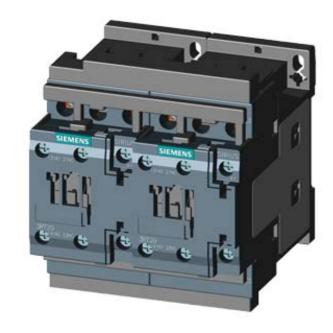
REV. COMB., AC3, 15KW/400V AC110V, 50/60HZ, 3-POLE, SZ SO SCREW TERMINAL ELECTR. AND MECH. INTERLOCK 2NO INTEGR.
