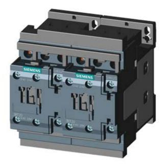
REV. COMB., AC3, 18.5KW/ 400V AC230V, 50/60HZ, 3-POLE, SZ S0 SCREW TERMINAL ELECTR. AND MECH. INTERLOCK 2NO INTEGR.
