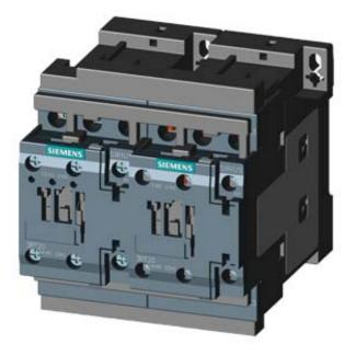
REV. COMB. W.I/O-LINK, AC3, 11KW/400V, DC24V 3-POLE, SZ S0 SCREW TERMINAL ELECTR. AND MECH. INTERLOCK 2NO INTEGR.
