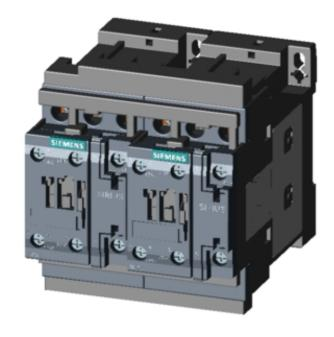
REV. COMB., AC3, 11KW/400V DC24V 3-POLE, SZ SO SCREW TERMINAL ELECTR. AND MECH. INTERLOCK 2NO INTEGR.
