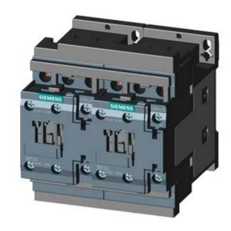
REV. COMB., AC3, 5.5KW/ 400V AC110V, 50/60HZ, 3-POLE, SZ SO SCREW TERMINAL ELECTR. AND MECH. INTERLOCK 2NO INTEGR.
