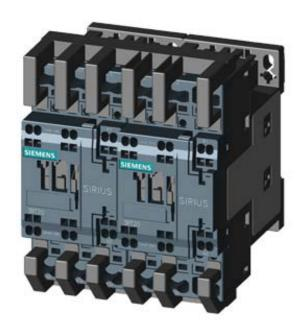
REV. COMB., AC3, 15KW/400V AC24V, 50/60HZ, 3-POLE, SZ SO SPRING-LOADED TERMINAL ELECTR. AND MECH. INTERLOCK 2NO INTEGR.
