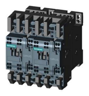
REV. COMB., AC3, 11KW/400V DC24V 3-POLE, SZ S0 SPRING-LOADED TERMINAL ELECTR. AND MECH. INTERLOCK 2NO INTEGR.
