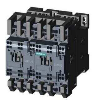
REV. COMB. W.I/O-LINK, AC3, 7.5KW/400V, DC24V 3-POLE, SZ S0 SPRING-LOADED TERMINAL ELECTR. AND MECH. INTERLOCK 2NO INTEGR.
