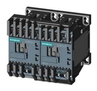
REV. COMB., AC3, 4KW/400V DC48V 3-POLE, SZ S00 SPRING-LOADED TERMINAL ELECTR. AND MECH. INTERLOCK
