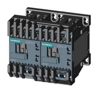
REV. COMB., AC3, 5.5KW/ 400V DC48V 3-POLE, SZ S00 SPRING-LOADED TERMINAL ELECTR. AND MECH. INTERLOCK
