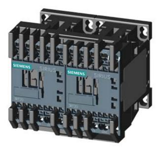
REV. COMB. AC3, 3KW/400V AC48V, 50/60 HZ, 3-POLE, SZ S00 SPRING-LOADED TERMINAL ELECTR. AND MECH. INTERLOCK
