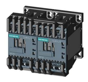
REV. COMB., AC3, 7.5KW/ 400V AC24V, 50/60HZ, 3-POLE, SZ S00 SPRING-LOADED TERMINAL ELECTR. AND MECH. INTERLOCK
