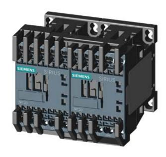
REV. COMB., AC3, 5.5KW/ 400V DC24V 3-POLE, SZ S00 SPRING-LOADED TERMINAL ELECTR. AND MECH. INTERLOCK
