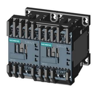
REV. COMB., AC3, 4KW/400V AC110V, 50/60HZ, 3-POLE, SZ S00 SPRING-LOADED TERMINAL ELECTR. AND MECH. INTERLOCK
