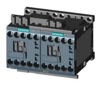
REV. COMB., AC3, 7.5KW/ 400V AC110V 50HZ/120V 60HZ 3-POLE, SZ S00 SCREW TERMINAL ELECTR. AND MECH. INTERLOCK
