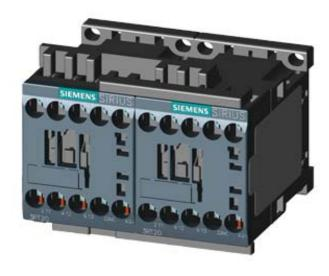
REV. COMB., AC3, 5.5KW/ 400V DC48V 3-POLE, SZ S00 SCREW TERMINAL ELECTR. AND MECH. INTERLOCK
