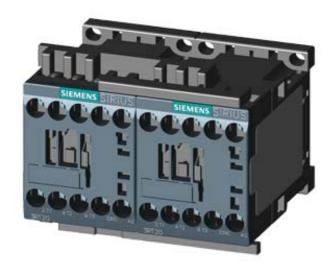
REV. COMB., AC3, 4KW/400V AC48V, 50/60 HZ, 3-POLE, SZ S00 SCREW TERMINAL ELECTR. AND MECH. INTERLOCK
