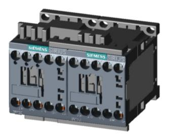
REV. COMB. W.I/O-LINK, AC3, 5.5KW/400V, DC24V 3-POLE, SZ S00 SCREW TERMINAL ELECTR. AND MECH. INTERLOCK
