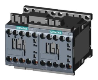
REV. COMB. W.I/O-LINK, AC3, 4KW/400V, DC24V 3-POLE, SZ S00 SCREW TERMINAL ELECTR. AND MECH. INTERLOCK
