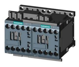
REV. COMB., AC3, 4KW/400V AC110V, 50/60 HZ, 3-POLE, SZ S00 SCREW TERMINAL ELECTR. AND MECH. INTERLOCK
