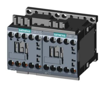
REV. COMB. W.I/O-LINK, AC3, 3KW/400V, DC24V 3-POLE, SZ S00 SCREW TERMINAL ELECTR. AND MECH. INTERLOCK
