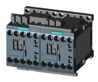
REV. COMB. AC3, 3KW/400V AC110V, 50/60 HZ, 3-POLE, SZ S00 SCREW TERMINAL ELECTR. AND MECH. INTERLOCK
